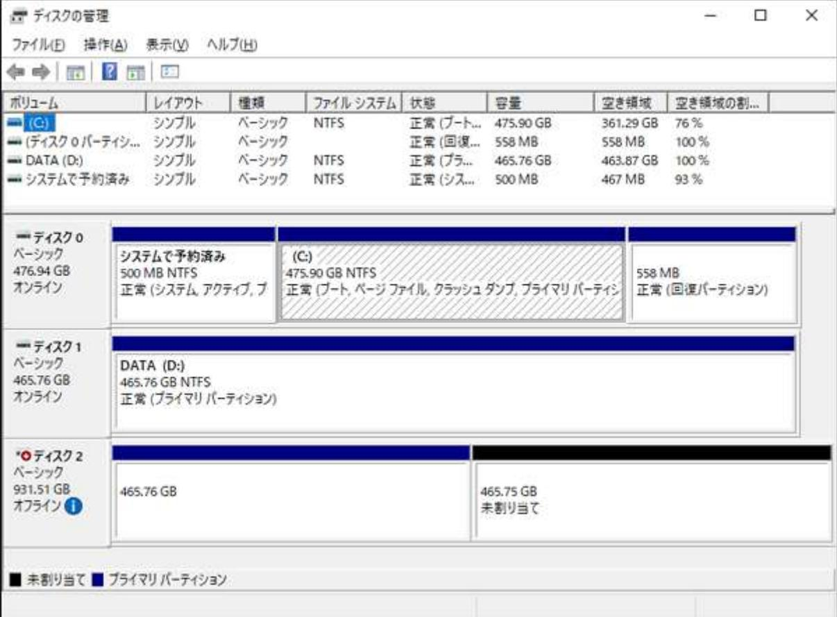
The screenshot shows the Windows Disk Management console. At the top, there is a menu bar with 'ファイル(F)', '操作(A)', '表示(V)', and 'ヘルプ(H)'. Below the menu bar is a toolbar with navigation and help icons. The main area contains a table of volumes and a detailed view of disks.
